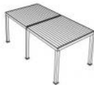
Type:E Two sets of pergola splicing: two sets side by side, sharing the middle column
